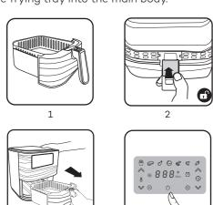
Please cover the Frying Basket Release Button with its cover when operating to avoid accidental pressing of the Button dropping the frying
